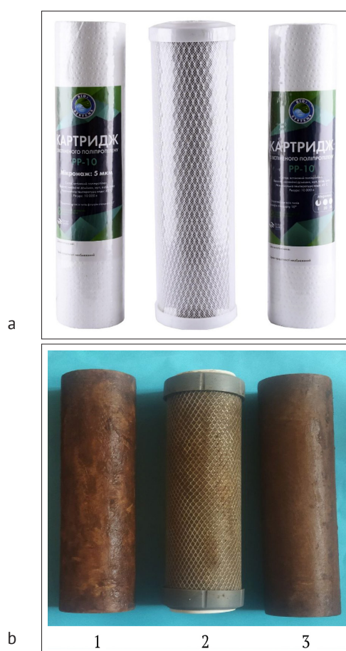
Figure 2. View of Ecosoft filters before and after use in a typical reverse osmosis plant for three months Source: developed by the author
