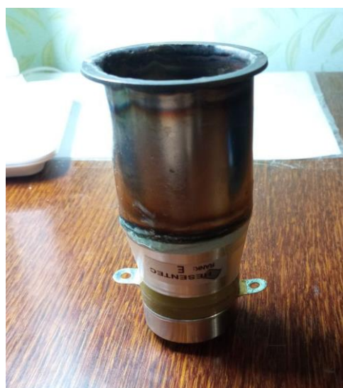
Figure 7. Experimental sample of ultrasonic system for extraction
