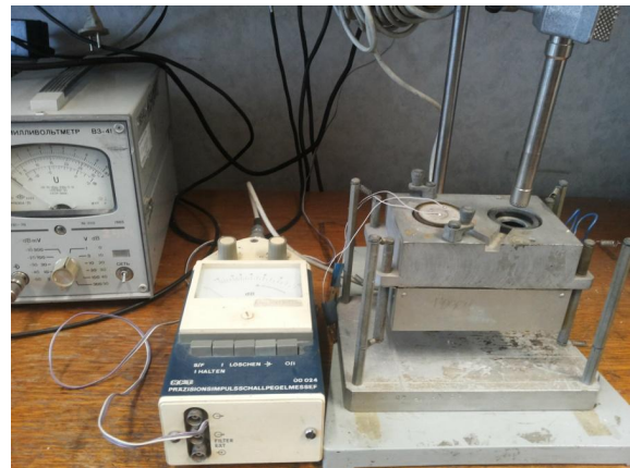
Figure 8 – Experimental stand with vibroacoustic chamber
