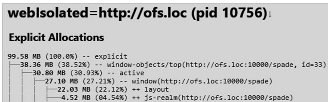
Figure 6. Detailed measurements of Firefox’s memory usage via “about:memory” special page (about:memory, n.d.) for the SPADE web interface tab
