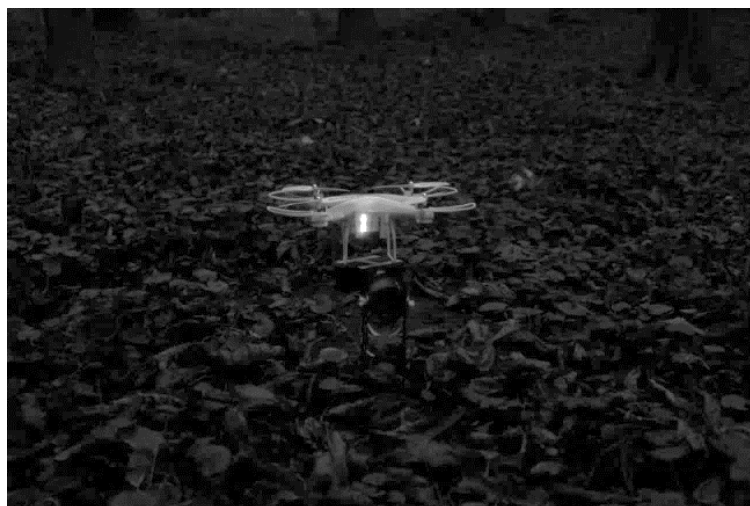
Figure 5. Drone on the landing platform during experiments with the proposed multi-beam drone positioning system
