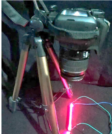
Figure 2. Optical setup for measurements of brightness distribution
